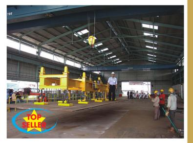
Latest technology for handling and lifting single plates of length upto 16mtr and width upto 4mtr. Completely eliminates the older electromagnetic conventional technology and its associated liabilities such as heavy electricity consumption, duty cycle adherence, battery backup, coil burnout and frequent maintenance.
