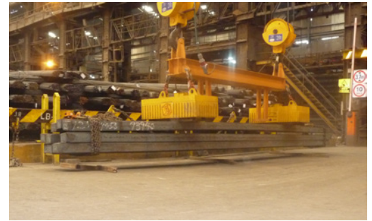
25 Ton Billet Lifter undergo load test
