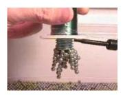
Finally, do the same thing with the third spool of 22 AWG wire. This spool will get much warmer. If it gets too hot to hold, disconnect the power supply from the spool of wire for a few minutes to give it time to cool off. Again, your goal is to find out the average number of BB's it can pick up.
