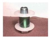
Connect the coil to the 5V power supply. If you have a multi-meter that can measure the
