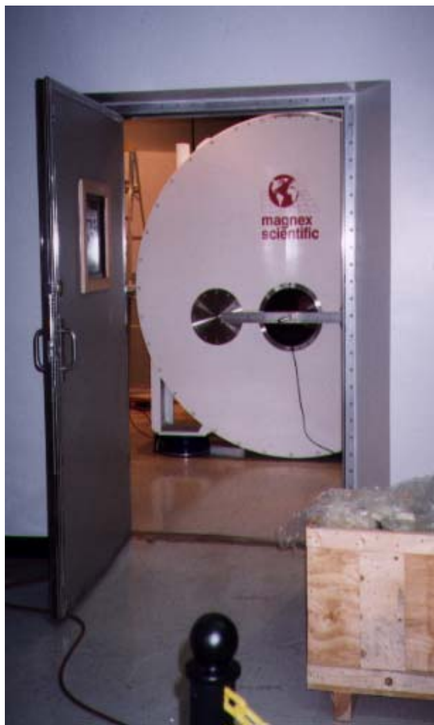
Magnex 500MHz (11.7T) 400mm bore magnet
